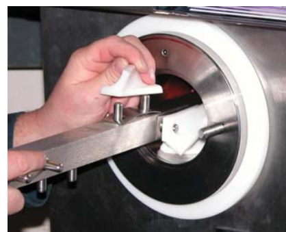
Figure 3-6 Installing Auger Blades
